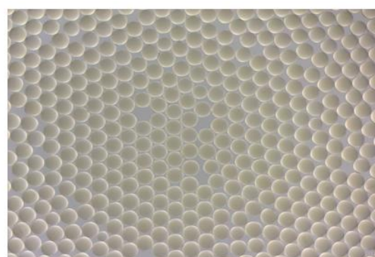
ZGA550G 凝胶强碱阴树脂高倍显微镜下形态
